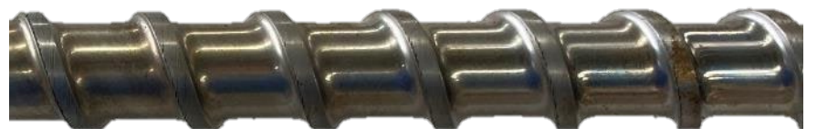
The same screw completely clean after purging with Asaclean™
