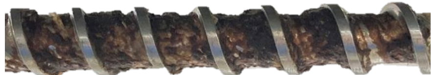
Carbonized resin generated by staying PA66-GF at 320°C for 90 minutes.
